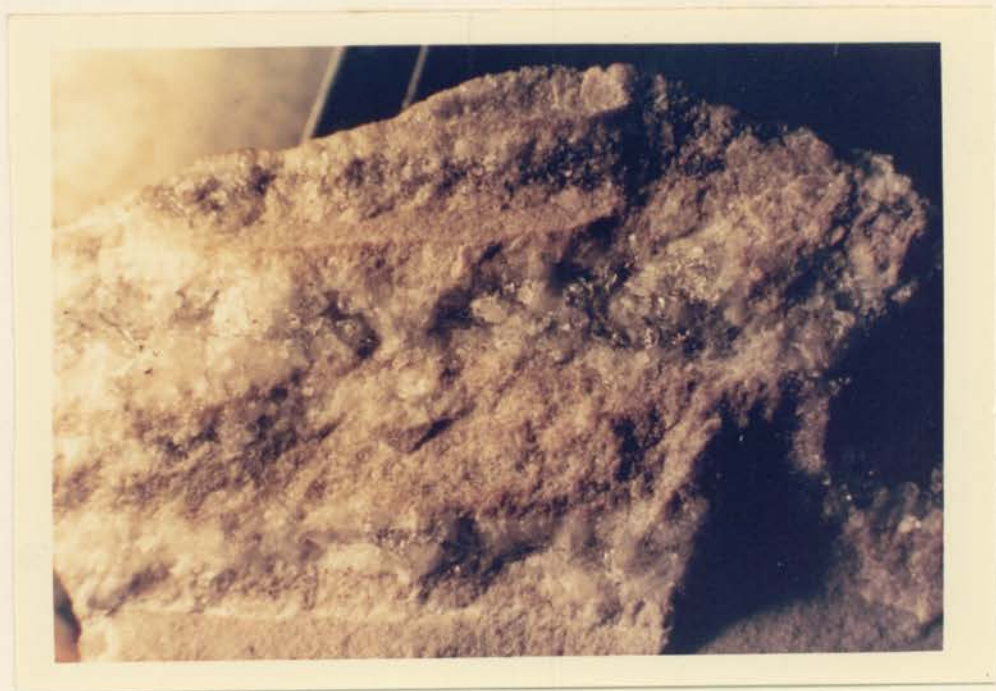
Photograph showing banded Limestone Core No. 3 at 2666 feet
