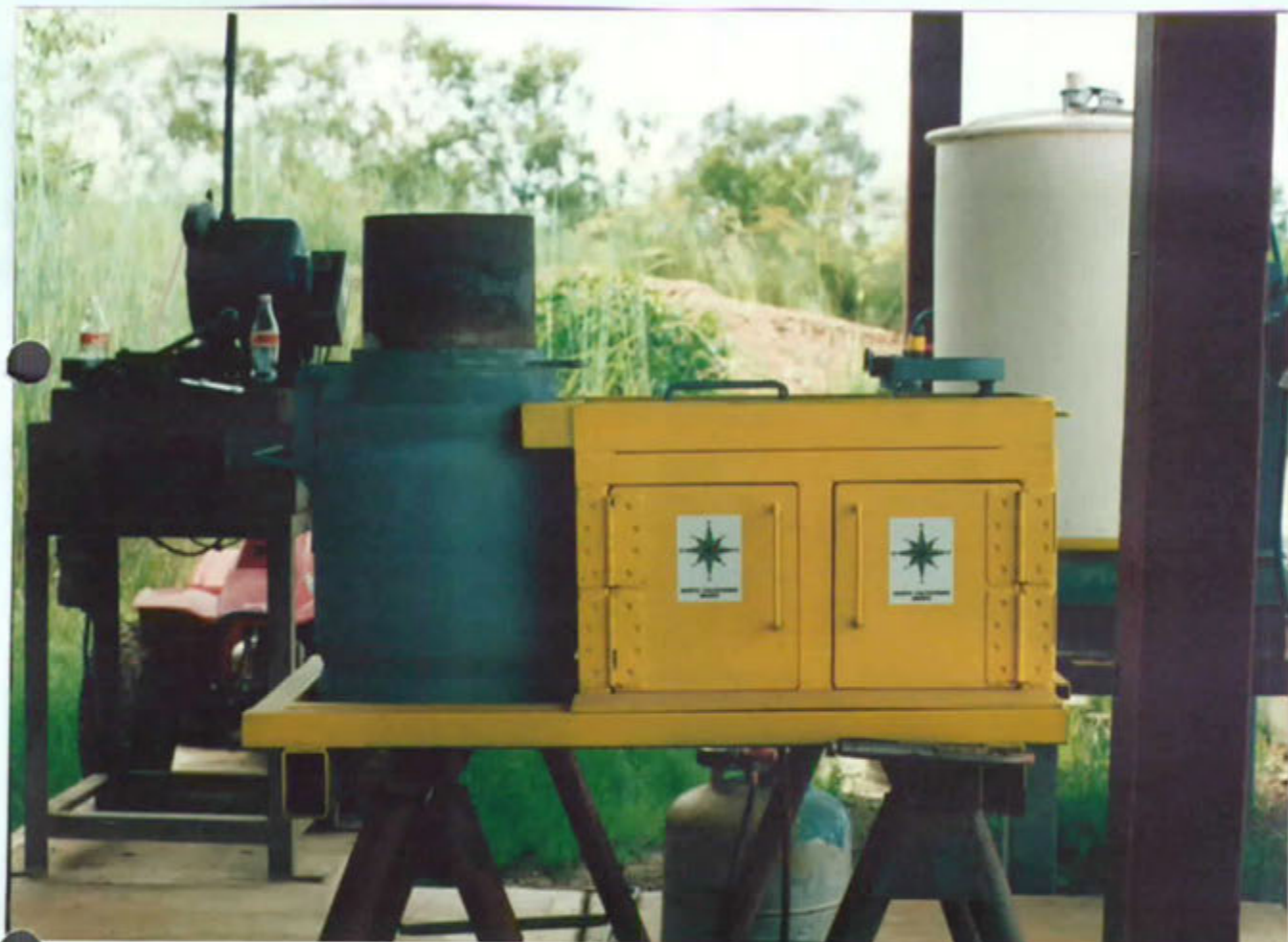
SMEETING FURNACE IN PLACE.
