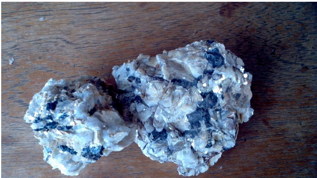
Photo 2 . Hand specimen of Sn-Ta-Nb ore from the tin field (at 130.79383 and -12.671268).
