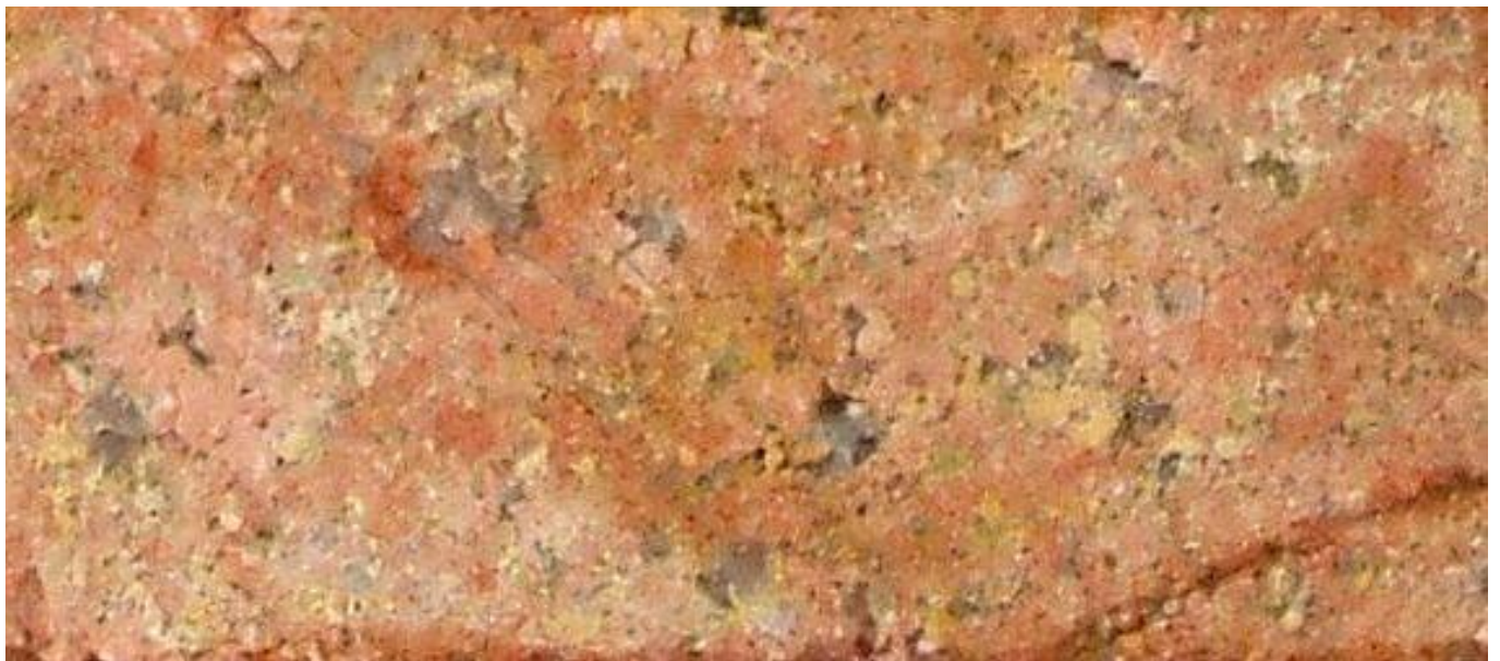
Figure 22. Specimen 171401. Fine grained granophyric granite. Rock slab. WOF c5.0cm.
