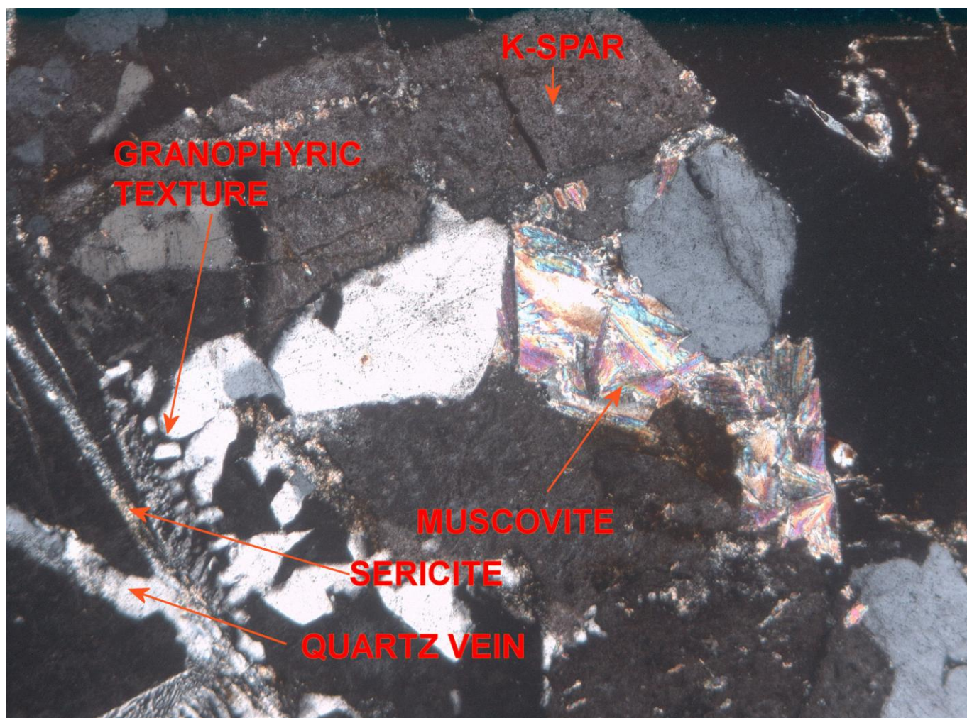
Figure 23. Specimen 171401. Granophyric texture and muscovite cluster. Thin section – crossed nicols. WOF c1.6mm.
