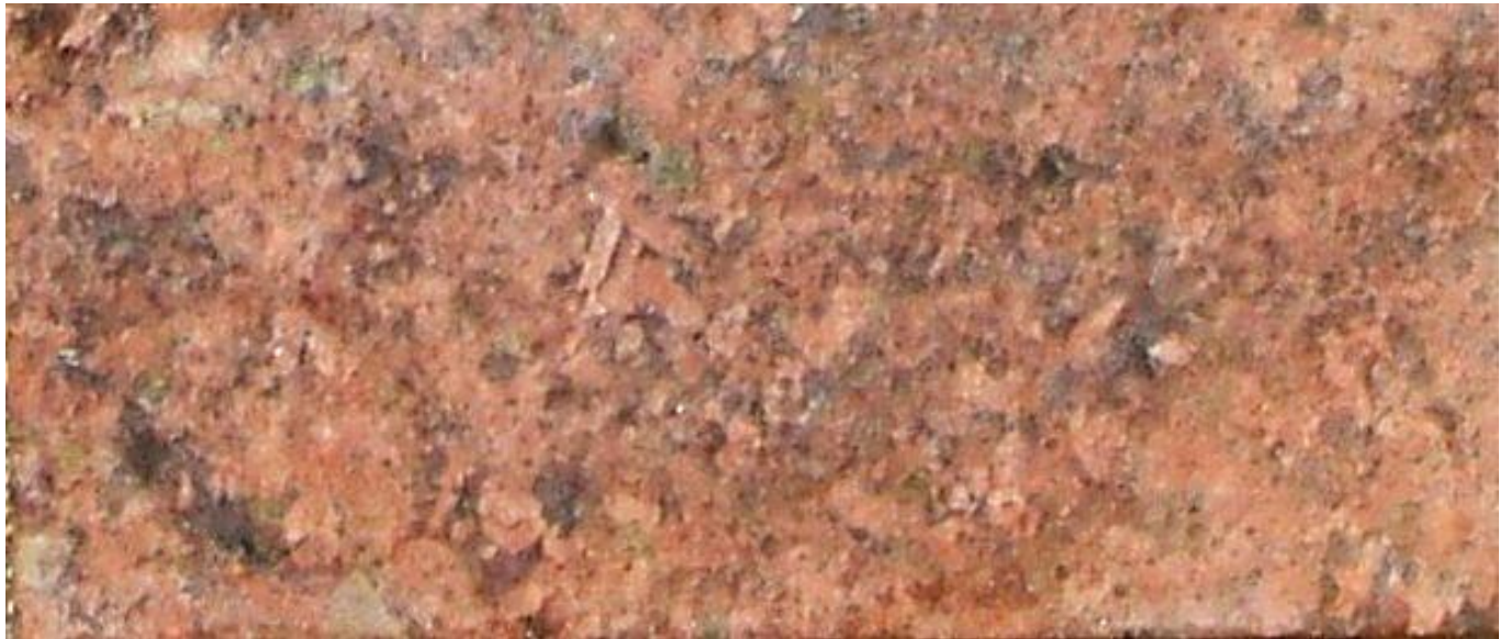
Figure 20. Specimen 171400. Medium to fine grained porphyritic/sericite granophyric granite. Rock slab. WOF c5.0cm.
