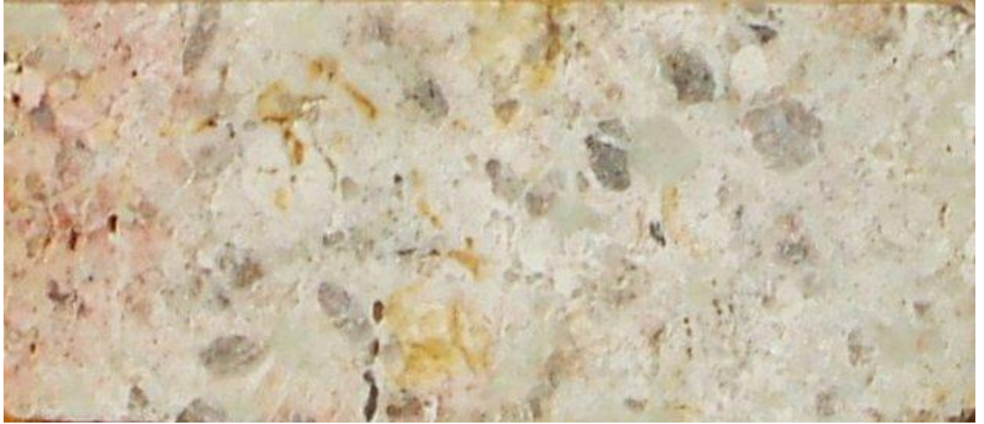
Figure 13. Specimen 171393. Medium to fine grained porphyritic granophyric granite – sericite/clay alteration. Rock slab. WOF c5.0cm.
