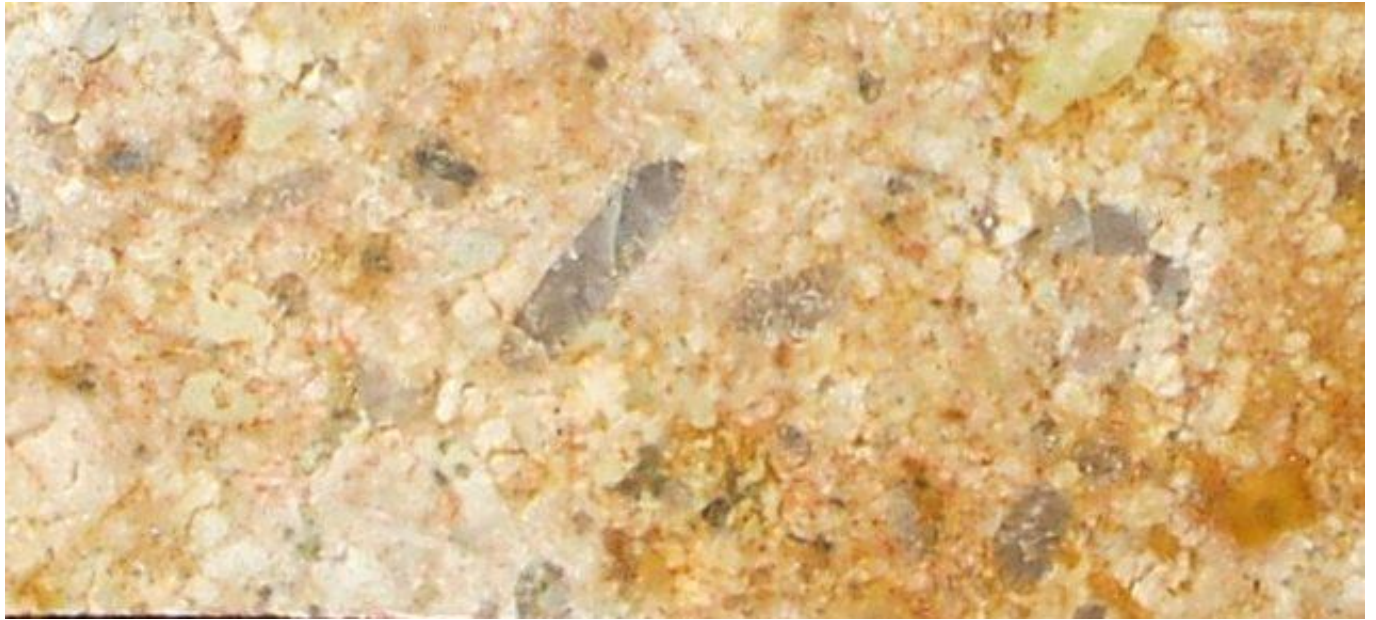
Figure 7. Specimen 171380. Medium grained porphyritic granophyric granite – sericite/clay altered. Quartz (dark), plagioclase (pale green), K-spar (pink). Rock slab. WOF c5.0cm.
