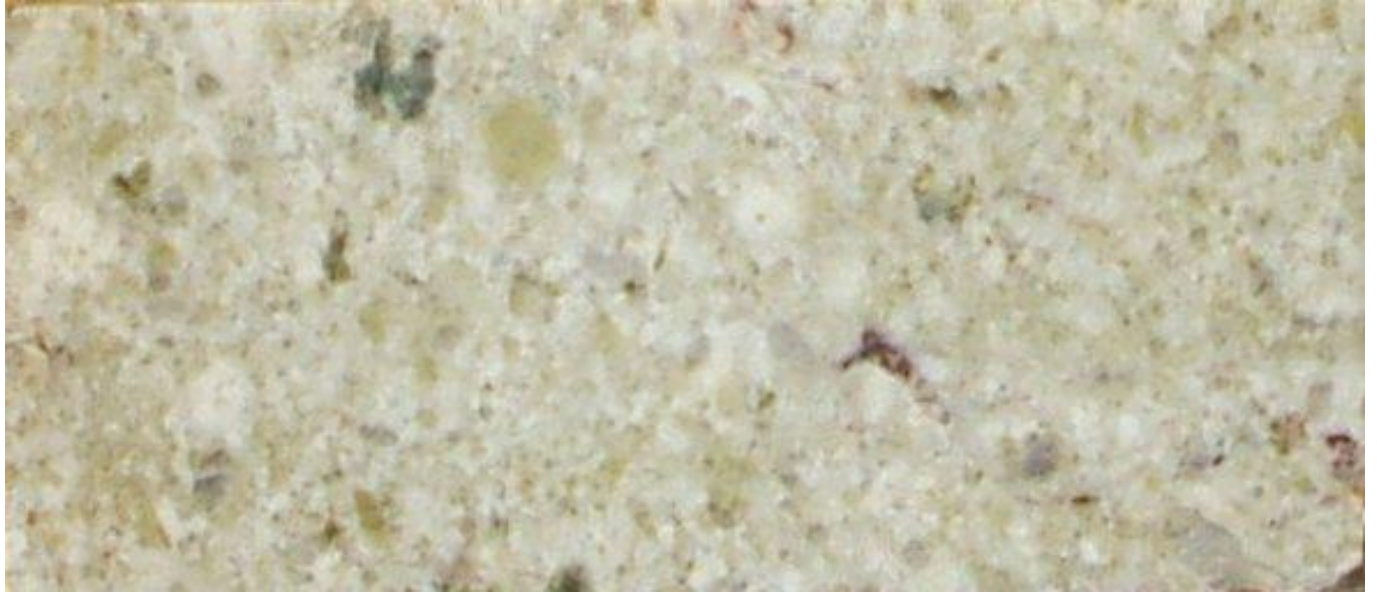
Figure 11. Specimen 171386. Clay/sericite altered medium to fine grained porphyritic granophyric granite. Rock slab. WOF c5.0cm.
