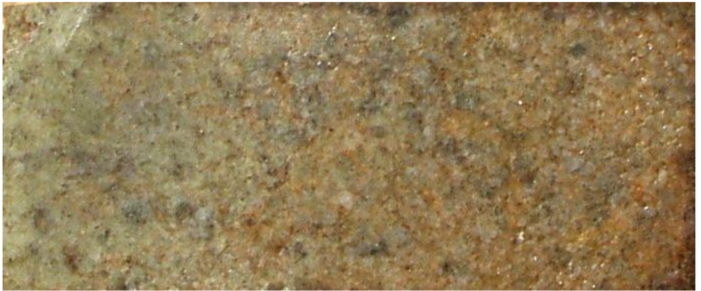
Figure 5. Specimen 171369. Sericitised (grey/green-left) fine grained slightly granophyric granite. Rock slab. WOF 5.0cm.
