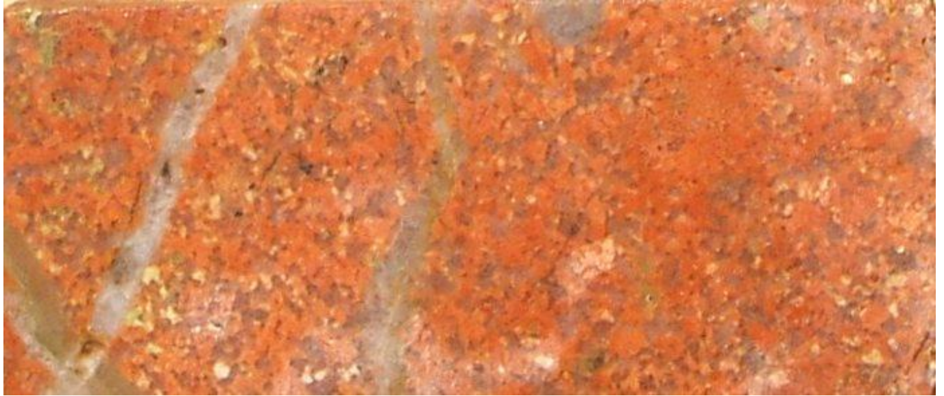
Figure 3. Specimen 171364. Fine grained, mildly porphyritic ( \pm granophyric) granite, with quartz veins. Rock slab. WOF c5.0cm.
