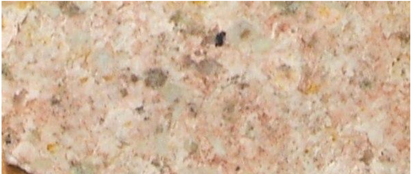
Figure 15. Specimen 171394. Medium to fine grained porphyritic granophyric granite – sericite/clay altered. Rock slab. WOF c5.0cm.
