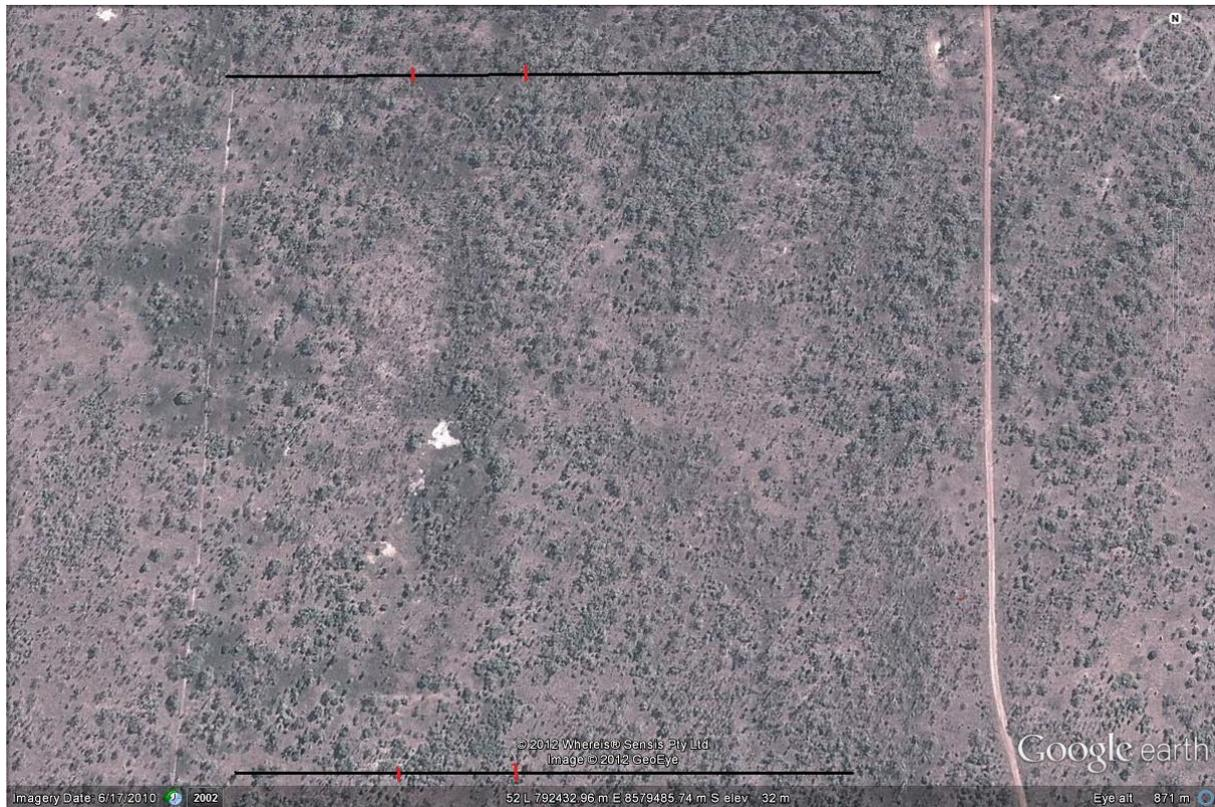
Google Earth image of relevant lengths of the two long drilling lines. Red strikes across the lines indicate the approximate positions of MGAC022 and MGAC023 on the top line and MGAC009 and MGAC010 on the bottom line. The geobotanical/lithological anomalous N – S striking feature that is related to the occurrence of vein quartz is clearly visible lying between these points.
