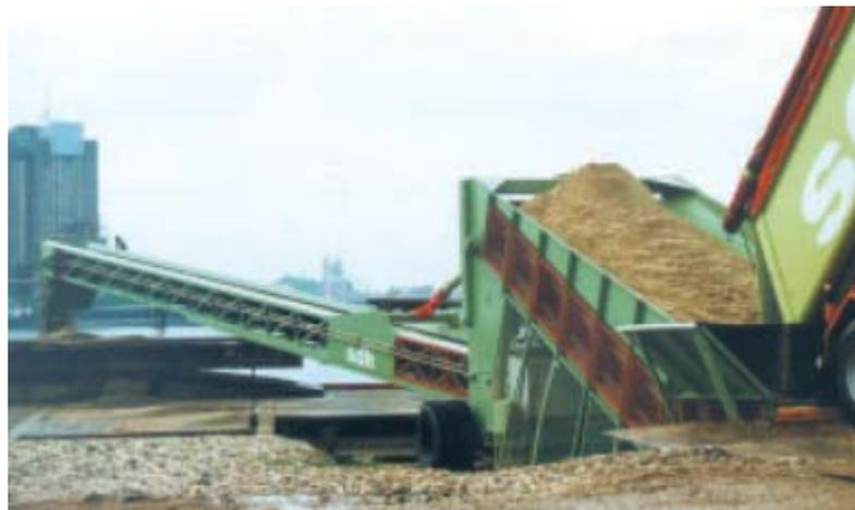
Figure 5 - Barge being loaded by mobile shiploader and truck
