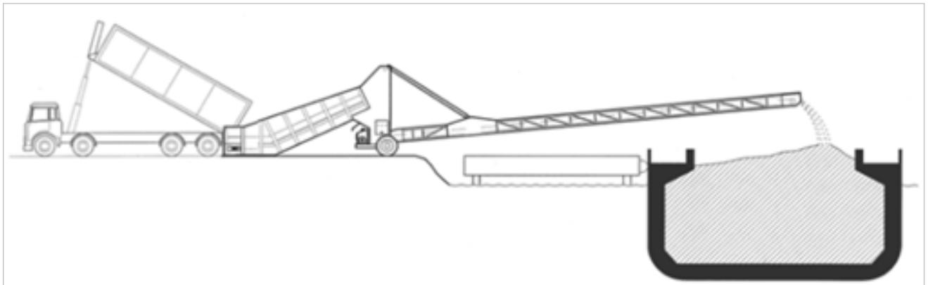
Figure 4 - Truck feeding the shiploading operation
