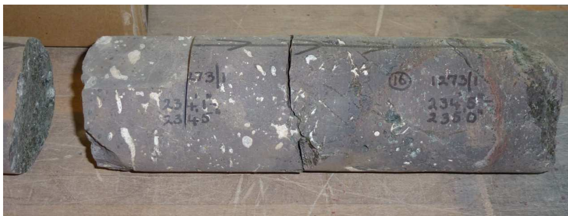
Figure 5 – A selection of the samples from Limbunya #1 core. Each sample contains 1.5 m of core, sampled as aggregated chips. Each box contains c. 25 m of core.
