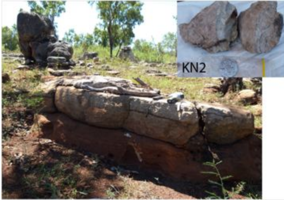
KN2 – Fine-grained buff/pale-grey “dirty” mottled limestone – partly recrystallised with degraded chalky/clay mottles, all highly calcareous.
