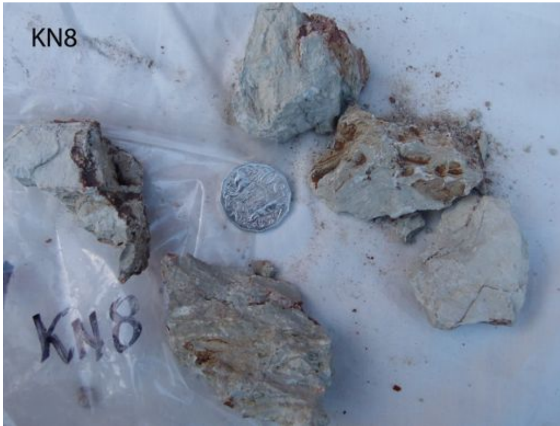
KN8 – Greeny-white chalky limestone. Layered in places, but not always in a laminar manner. The greeny layers are more tenacious whilst the whiter layers are more chalky and powdery. Occasional ferruginous lenses occur throughout. Recrystallisation is present, but is very minor. Both layer-types are calcareous.
