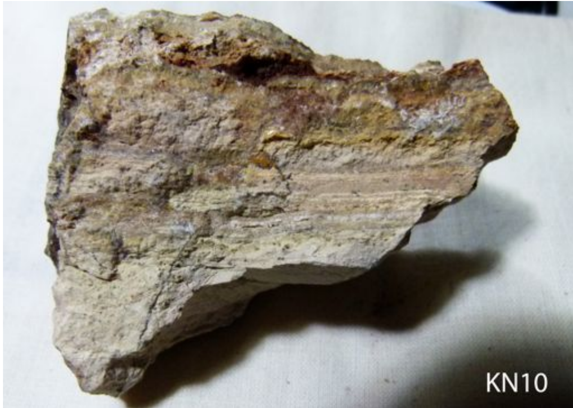
KN10 – Layered pinky/yellow “dirty” limestone. Highly laminated fine-grained to medium-grained limestone that has been subjected to a considerable degree of fluid movement commonly manifesting itself as layer-parallel calcite veining. Iron oxide (occasional orangey lenses) is also deposited along some beds that have clearly been subject to meteoric fluid flow. All layers are calcareous.
