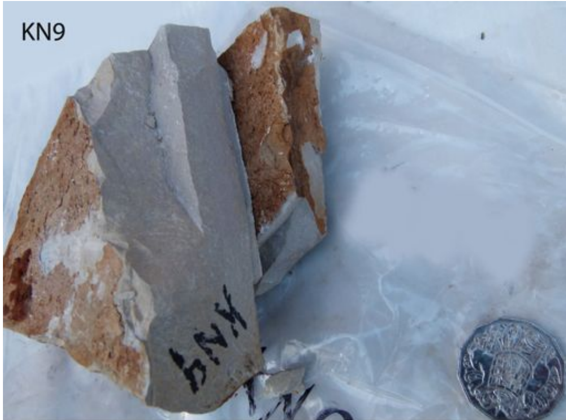
KN9 – Pale pink “clean” laminated limestone. Layers vary considerably in thickness but are clearly sedimentary laminae. Grains are generally very fine, almost micritic and very tenacious despite little evidence of recrystallisation. Ferruginisation is evident, but appears to be restricted to groundwater pathways (fractures and unloading joints).
