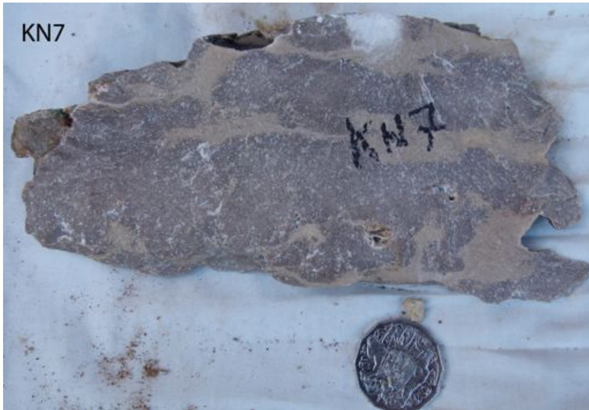
KN7 – Buff/Grey purpley-mottled “dirty” limestone. Colour differentiation appears to be broadly due to a sedimentary layering but appears to have undergone some level of differential recrystallisation associated with grain-size differences. The buff layers appear to weather in a more recessive manner than the gray/purple. All are highly calcareous.
