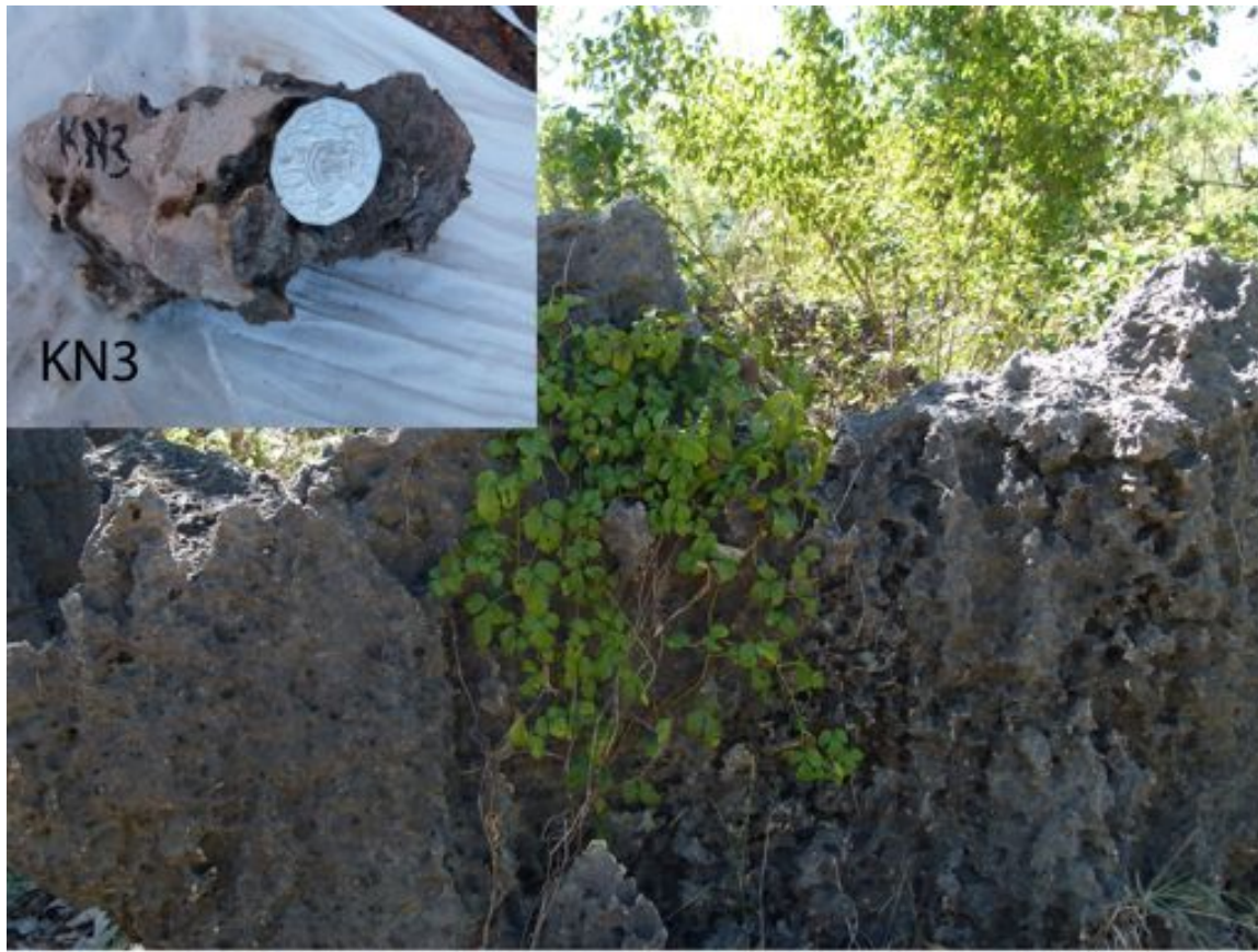
KN3 – Pinky “dirty” limestone with dark grey surface-colouring and heavy surficial karsting. Small specks of black possibly manganese present near the surface. Fair degree of recrystallisation becoming more evident away from the “degraded” surface. Highly calcareous throughout.
