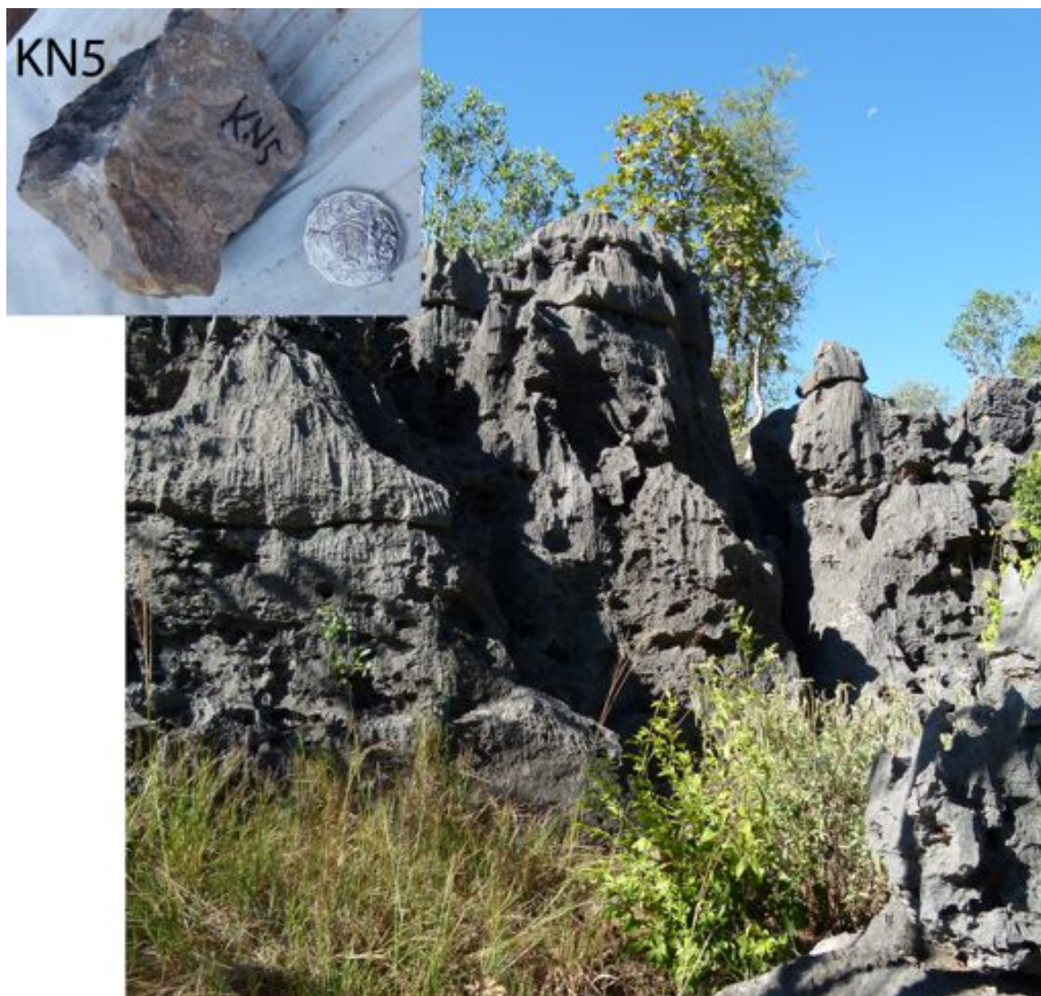
KN5 – Bedded/brecciated limestone/shale - buff/grey in colour internally, but dark grey surfacial colouration. Layers differ considerably in grain-size and composition, with the finer-grey limestone layers being highly-calcareous and the (mostly coarser) buff-coloured layers only mildly so.
