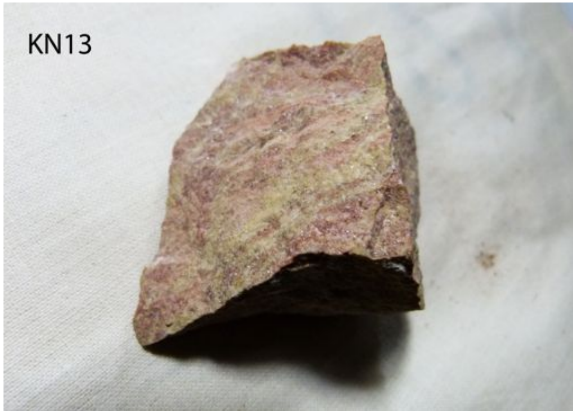
KN13 – Pink/Pale green stromatolitic (?) limestone. Predominantly layered, alternating between pink and pale green layering, but generally not laminar and commonly appears to form stromatolitic patterns that may be seen more clearly on weathered surfaces. Degree of recrystallisation is high and results in a highly tenacious unit.
