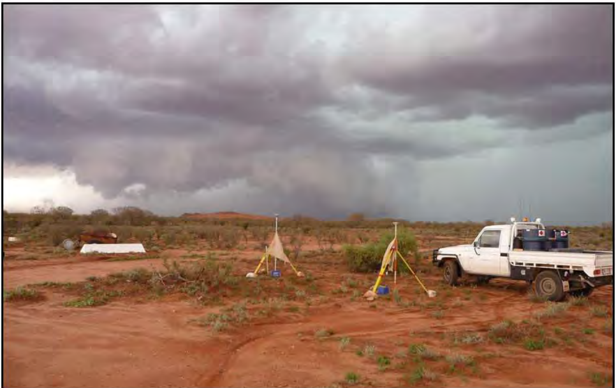
Photo 8: Post process GPS base setup at Kulgera Airfield.
