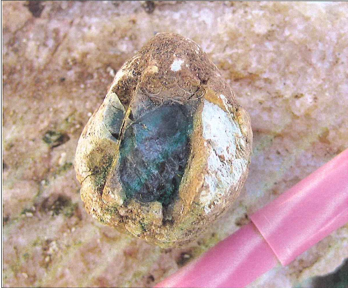
Figure 8. One of the strongly radiogenic concretions found in the soil near the site of PNC Trench 4 (immediately north of the road) at Yambla. This concretion is approximately 3 cm in diameter and contains what appears to be uraninite surrounded by clay alteration. Other concretions contain mm scale “veins” of secondary minerals after uraninite.
