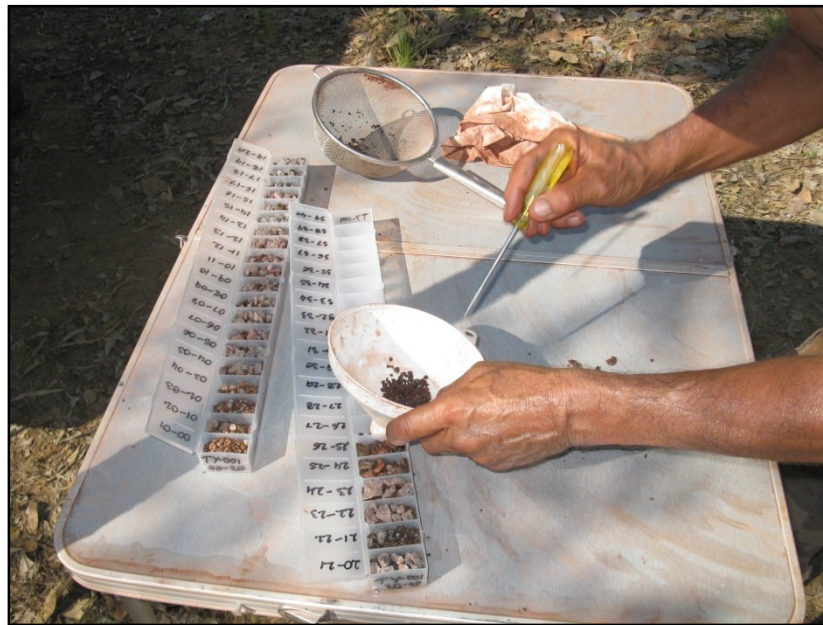
Photo 5: Placing sieved/washed drill cuttings into chip tray
