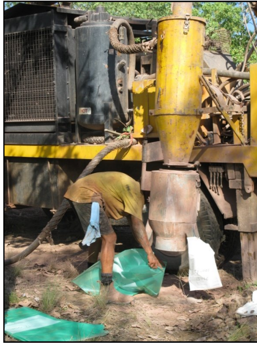
Photo 3: Sample cyclone, splitter & sample bags
