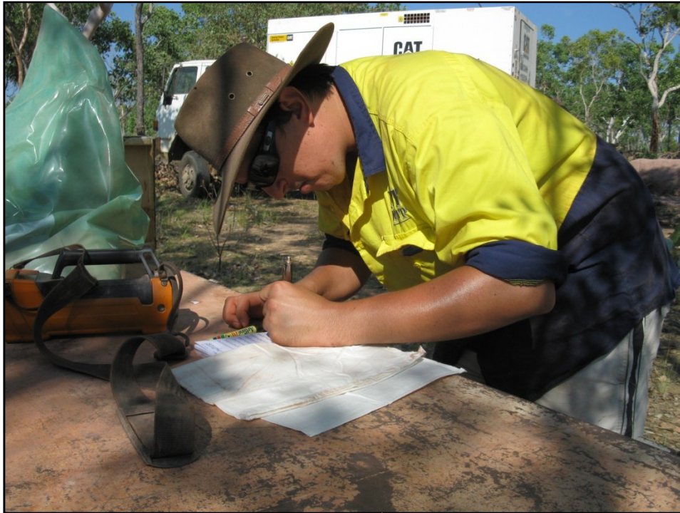
Photo 7: Spectrometer assay of one-metre bulk sample and data recording
