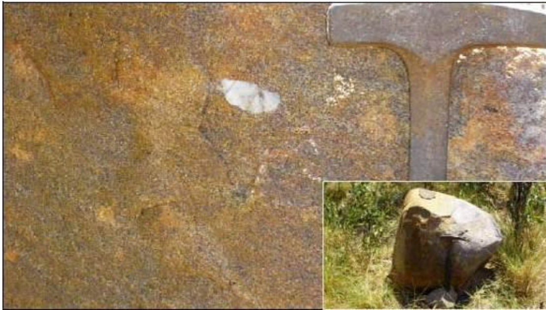
G5 Westmoreland Conglomerate – coarse grain ferruginous pebbly lithic quartz sandstone minor fine well rounded quartz cobbles. 717000e 8055310n GDA94_UTM53 (γ: 84 cps).
