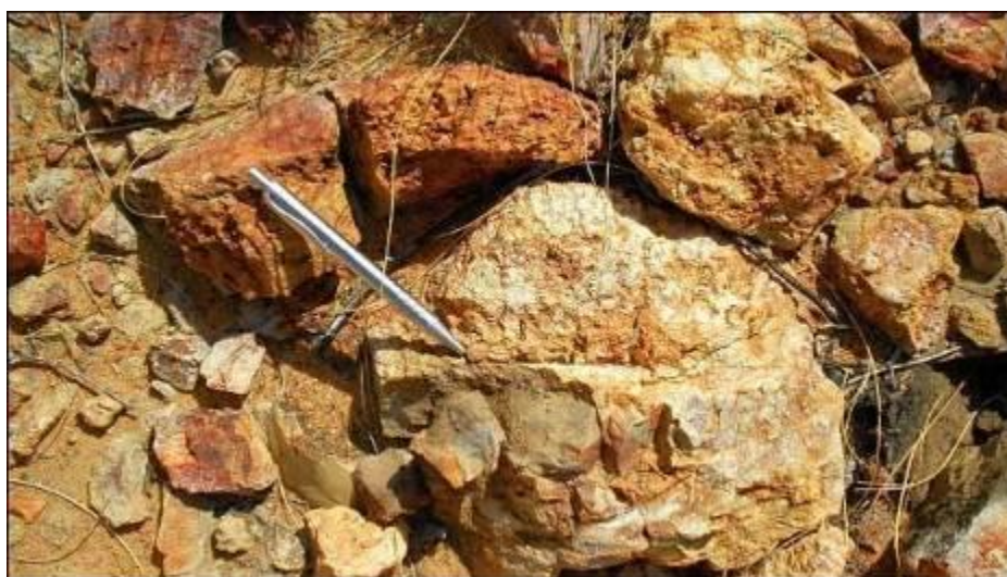
G26 Fine to coarse grained sheared metasediments (-Pbb) with quartz veins and boudins? - sheared conglomerate? 702005e 7990660n. Dip 56 / 250 (<120 cps).
