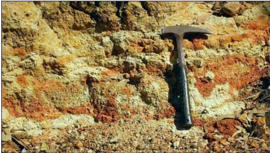
G6 Fine to coarse sandstone and interbedded pebble conglomerate (ferrug. saprolite). Bukalara Sandstone exposed in creek bank. 707350e 8038330n (γ: 164 cps). Flat-lying.
