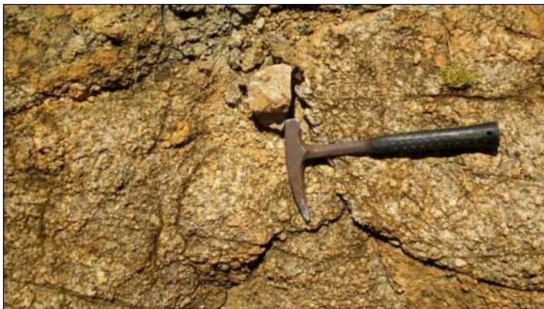
G15 Very coarse grained inequigranular granite. 716640e 8032250n ( \gamma : <250 cps).
