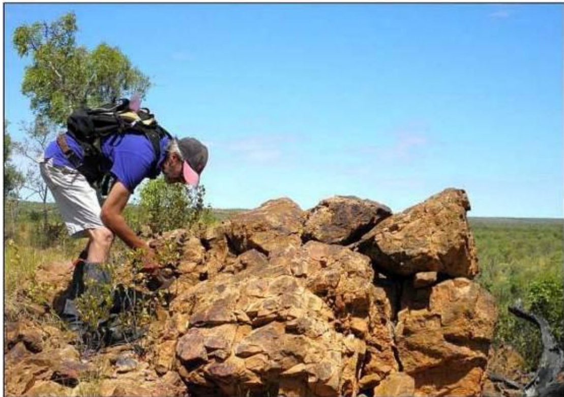
G29 Mullera Formation (-Psl) or (-Plm?) – medium to coarse grained matrix supported pebbly sheared meta-sandstone, minor quartz veining. Dip vertical 710175e 8014310n (84 cps).
