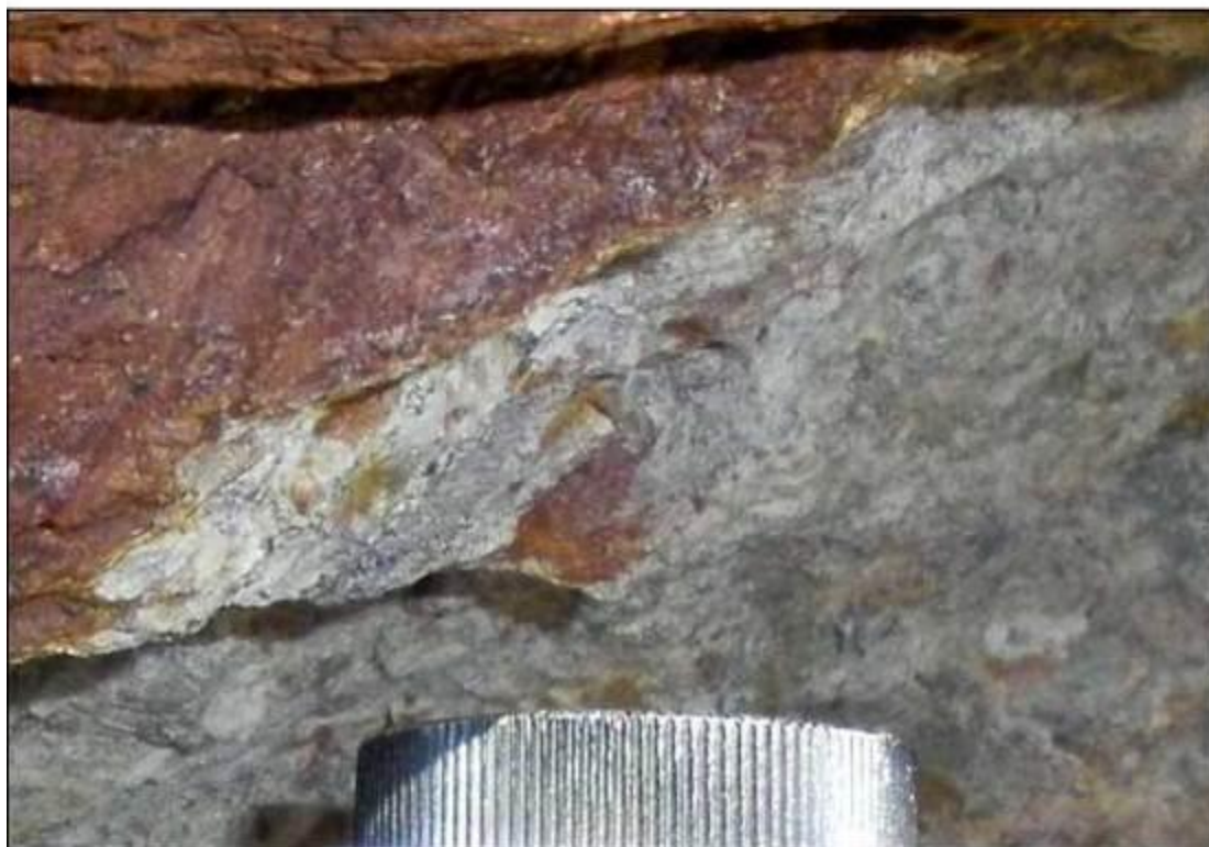
G18 Anomaly 1 float vein material. Scintillometer > 9999 cps.
