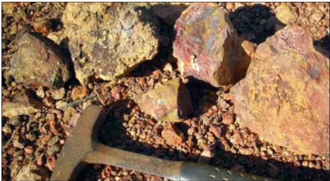
G12 Strongly ferruginised (laterite) medium coarse grained inequigranular granite hill. 707780e 8035713n (212 cps).
