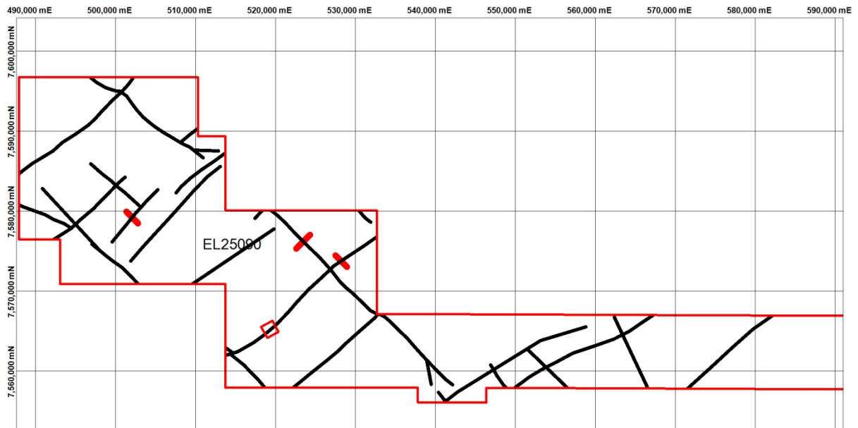
Figure 3: Faults interpreted from worm processing of detailed gravity survey as black lines, and soil sampling traverses as red lines, on a map of EL25090.
