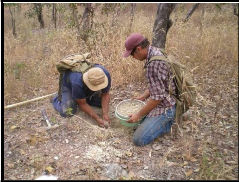
Collecting & sieving soil samples in the field Plate 4
