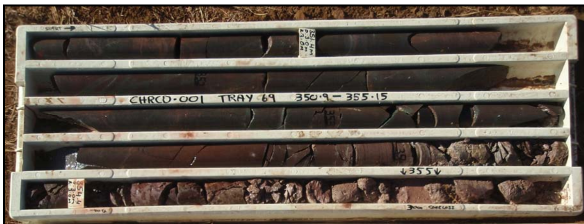
Plate 5 CHRCD001-Core samples from 350.90- 355.15m, the broken reddish brown clay / siltstone zone can be seen in the bottom 2 rows
