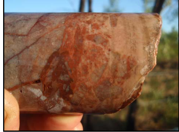
Plate 7 Silicified Westmoreland Conglomerate-Quartz, hematite veining in a crackle breccia setting (CHRCD001)
