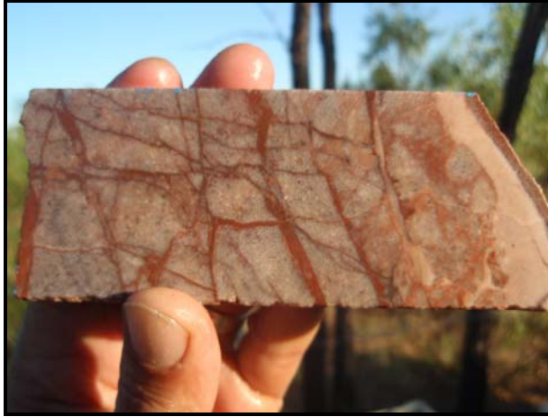
Plate 6 Silicified Westmoreland Conglomerate- Stockwork hematite veining with jasperite textures (CHRCD001)
