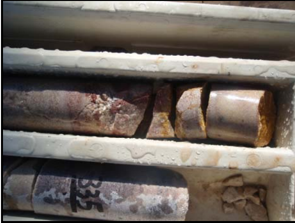
Plate 10 Westmoreland Conglomerate unit- Broken zone at 334m with slightly anomalous gamma readings observed in CHRCD002
