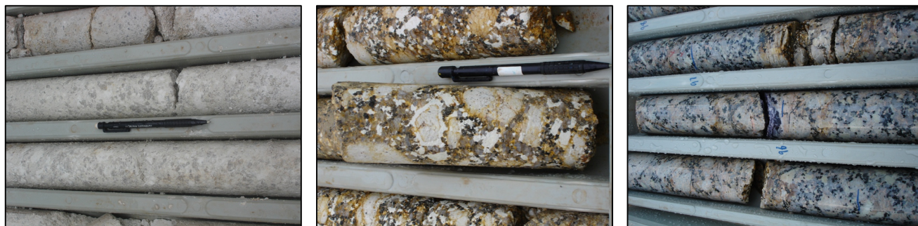
Figure 3. Weathering/alteration profile documented from 2008 drilling; (a) Heavily kaolinised, (b) moderately altered and (c) “fresh” granites.
