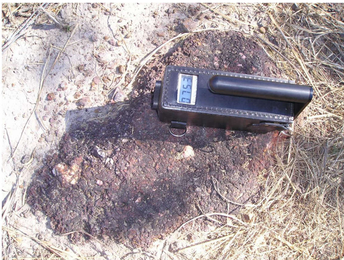
Figure 5: Subcrop of lateritised fluvial hardpan. Scintillometer is reading 753 cps (counts per second)
