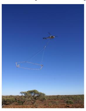
survey used the SkyTEM system with a terrain clearance of 30 metres. The traverse line spacing was 150 metres. Details of the survey are given in the logistics report in appendix 3. The data are detailed in appendix 4.
