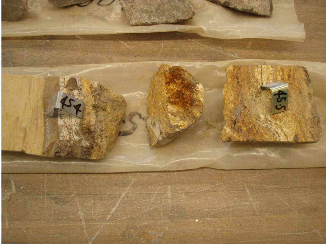
Figure 5. BMR Hay River 11A core. The white band at marker 45.4m (metre 118.4 of the composite section) is phosphorite containing 313 ppm uranium. The dark band immediately above (to the left) contains 0.52% zinc.
