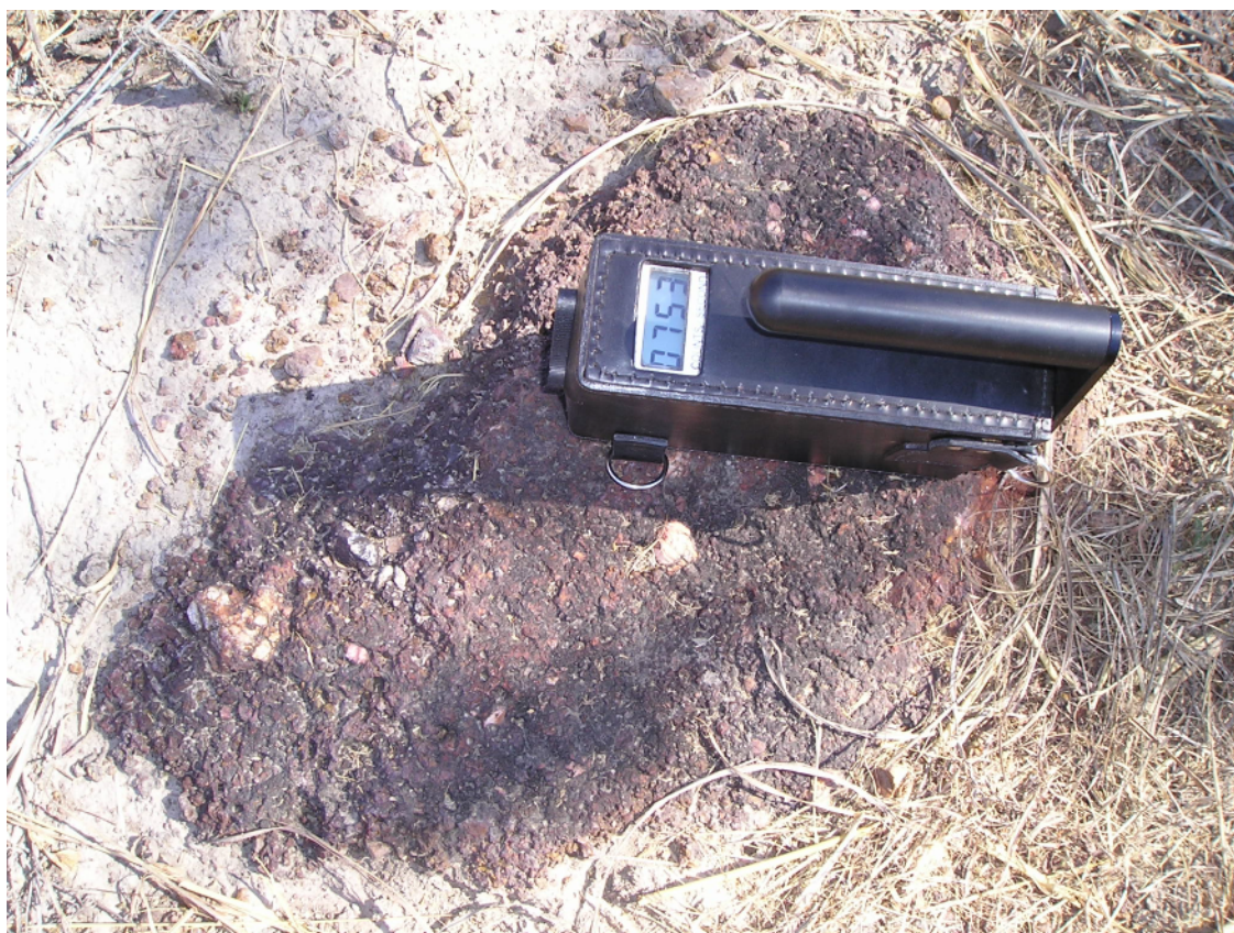
Figure 8: Subcrop of lateritised fluvial hardpan. Scintillometer is reading 753 cps (counts per second)
