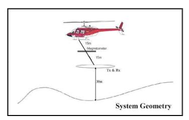
The transmitter / receiver configuration has a nominal 35 metre terrain clearance. Helicopter survey speed is between 35 and 45 knots, resulting in an along line sample interval of between 8 and 10 metres for the acquired EM data. The primary waveform used is a 25% duty cycle square wave, with a 5ms current on-time (including 1ms cosine ramp on) and 15 ms current off-time. The receiver measures the Earth's response during the current-off time. The maximum pulse current used is 320 Amps.
