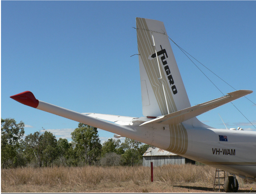
Figure 3a Aircraft with rear stinger instrument mount
