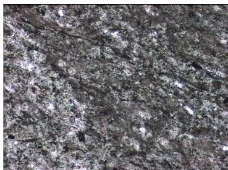
Left. 26027.01. 1200 \mu\text{m} ppl. Fragmental texture and lamination ghosted secondary feldspar or cordierite crystals.
