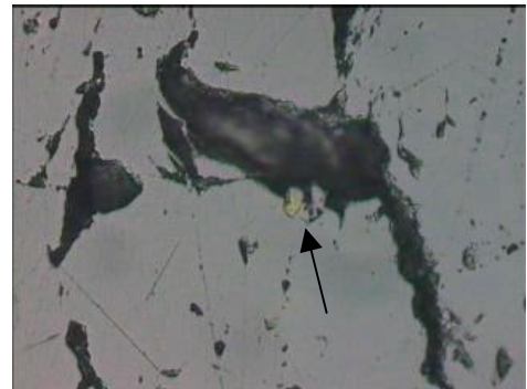
Left. 26027.02. Thermally and tectonically overprinted quartz + arsenopyrite cemented breccia in mudstone. Arsenopyrite is host to a gold inclusion. Right. 26027.02. Native gold inclusion within arsenopyrite. 120 \mu\text{m} . rl/ppl.
