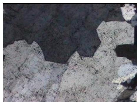
Left. 26027.03. Second stage quartz veining hosted by basalt.
