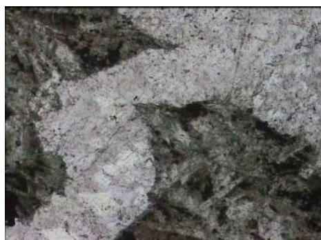
Left. 26027.03. Folding of early vein cross-cut by later quartz vein style. 1200 \mu\text{m} . ppl.
