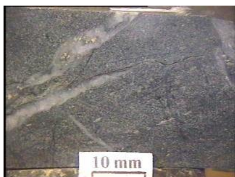
Left. 26027.03. Second stage quartz veining hosted by basalt.
