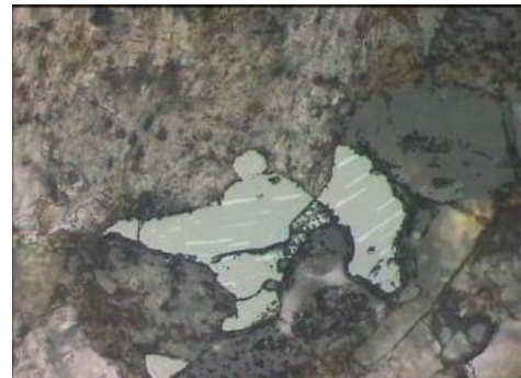
Left. 26025.01. Ilmenite intergrown with primary silicate minerals. 300 \mu\text{m} . ppl/rl. Right. 26025.02. Magnetite with hematite exsolution lamellae in primary mineralogy. 300 \mu\text{m} . ppl/rl.
