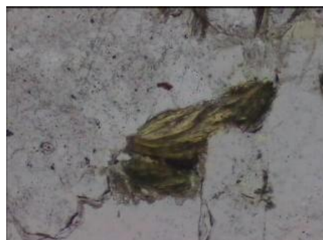
Left. 26025.05. Halite bearing aqueous liquid-rich inclusions occurring with less abundant gas-rich inclusions. 120 µm. ppl. Right. 26025.11. Preserved biotite interstitial to quartz of quartz veining. 600 µm. ppl.
