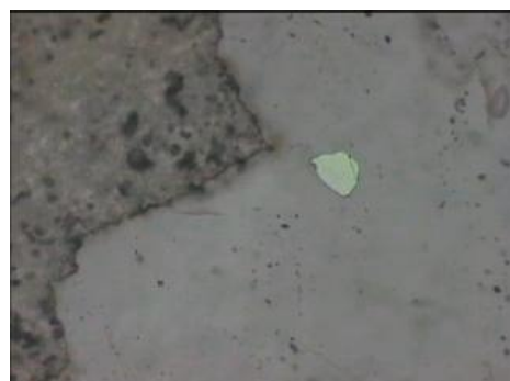
Left. 26025.04. \text{CO}_2 -rich inclusions in primary quartz. 120 \mu\text{m} . ppl. Right. 26025.04. Chalcopyrite inclusion in primary quartz. 120 \mu\text{m} . ppl/rl.
