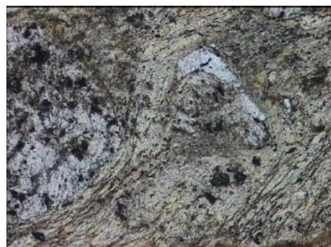
Left. 26025.08. Fragments of granitoid rock, quartz and K-feldspar enclosed within anastomosing sericitic matrix (after plagioclase) defining cataclastic texture. 1200 \mu\text{m} . cpl. Right. 26025.08. as above. 1200 \mu\text{m} . ppl.
