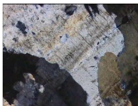
Left. 26025.05. Late quartz veinlet traversing cataclastic texture and strong illitic clay alteration. 1200 \mu\text{m} . ppl. Right. 26025.11. Shear fabric and fluid inclusion trails overprinting igneous style quartz veining. 1200 \mu\text{m} . cpl.
