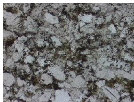
Left. 26025.07. Drill chips comprising metamorphosed sedimentary lithologies. Right. 26025.07. Relict fragmental texture in metamorphosed sedimentary rock. 1200 \mu m. ppl.
