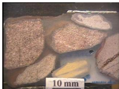
Left. 26025.07. Drill chips comprising metamorphosed sedimentary lithologies. Right. 26025.07. Relict fragmental texture in metamorphosed sedimentary rock. 1200 \mu m. ppl.
