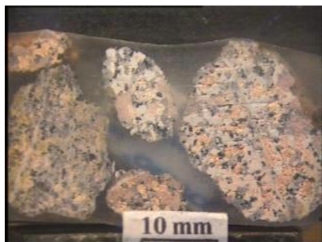
Left. 26025.09. Relatively coarser grained textures and pale red-brown K-feldspar. Right. 26025.09. Abundant quartz enclosing ghosted euhedral plagioclase and interlocking with K-feldspar and brown biotite. 1200 \mu\text{m} . ppl.
