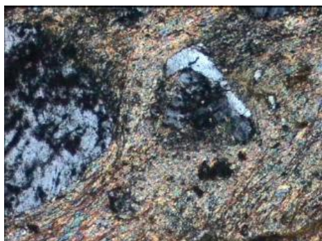
Left. 26025.08. Fragments of granitoid rock, quartz and K-feldspar enclosed within anastomosing sericitic matrix (after plagioclase) defining cataclastic texture. 1200 \mu\text{m} . cpl. Right. 26025.08. as above. 1200 \mu\text{m} . ppl.
