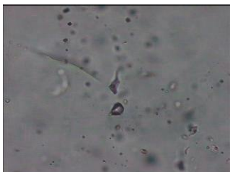
Left. 26025.04. \text{CO}_2 -rich inclusions in primary quartz. 120 \mu\text{m} . ppl. Right. 26025.04. Chalcopyrite inclusion in primary quartz. 120 \mu\text{m} . ppl/rl.
