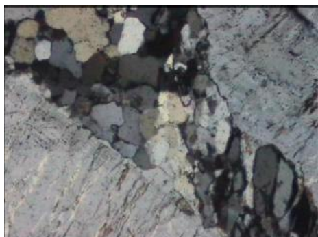
Left. 26028.08. Recrystallised quartz + K-feldspar veinlet. 600 µm. cpl.
