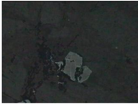
Left. 26028.01. Ilmenite inclusions in feldspar and quartz. 300 µm rl/ppl.
