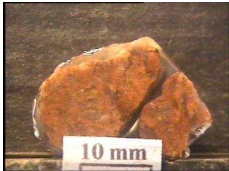
Left. 26028.01. Quartz and K-feldspar rock, with K-feldspar impregnated with hematite.
