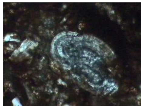
Left. 26028.07. Typical fragmental texture with quartz and ghosted feldspar detrital fragments. 300 \mu m. Right. 26028.07. Possible bioclast fragment amongst detrital fragments. 300 \mu m. ppl.
