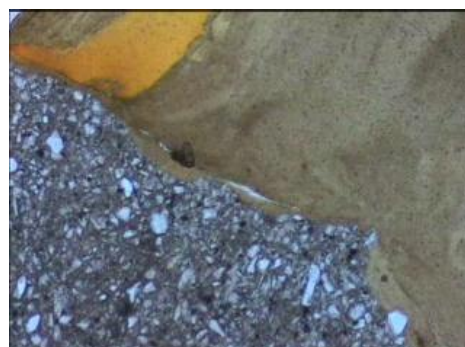
Left. 26028.06. Weathered sediment host to low temperature vein. Right. 26028.06. Banded kaolin, goethite and amorphous silica vein in fragmental textured wallrock. 1200 \mu m. ppl.
