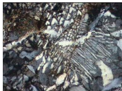
Left. 26028.03. Graphic intergrowths...300 \mu\text{m} . cpl. Right. 26028.21. Graphic intergrowths...1200 \mu\text{m} . cpl.
