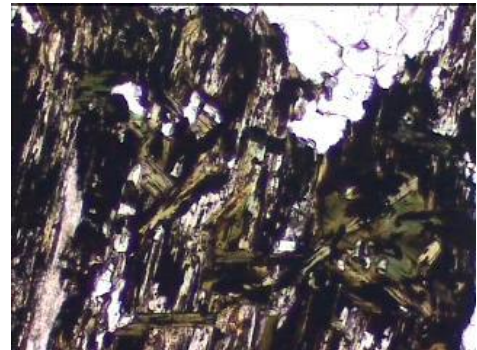
Left. 26028.01. Ilmenite inclusions in feldspar and quartz. 300 µm rl/ppl.
