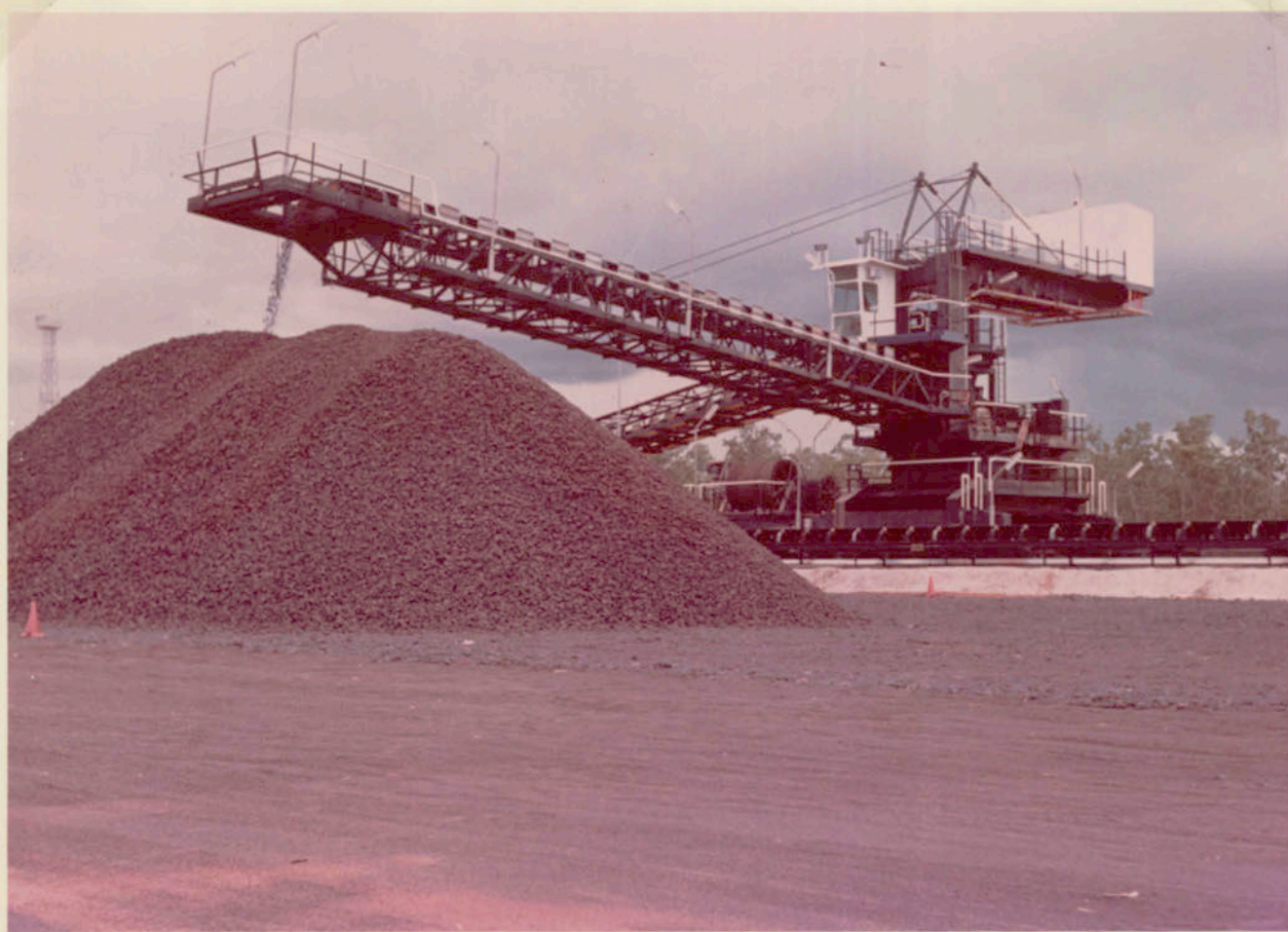
New stacker in operation. Ore from stockpile is reclaimed by bucketwheel reclaimer (not shown) for loading into ships.
