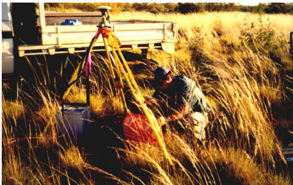
Figure 3 Dave Daish from Daishsat Pty Ltd of Murray Bridge, South Australia collecting gravity readings along a north-south profile traverse in EL 8882.
