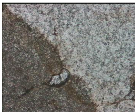
Plate 7 a & b. TLAC006/6-14 Fragment of igneous (granitoid) framework quartz (right) enclosed by crustiform banded silcrete lithology comprising cristobalite, kaolinite and smectite (width of view is approx. 1300 \mu\text{m} ).
