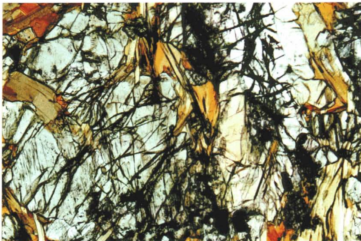
MC - DM1. Biotite olivine clinopyroxenite with pale green, moderately altered clinopyroxene, generally fine-grained biotite and olivine (clear) with abundant fractures and opaque inclusions. Plane light. FOV = 2.6 mm.
