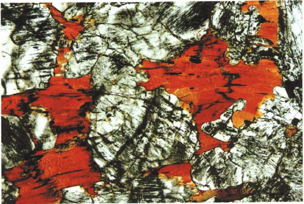
MCDDH2 - 40.5m. Olivine biotite clinopyroxene with coarse-grained, pale green clinopyroxene moderately to strongly altered and containing very fine-grained opaque and tremolite. Red-brown biotite is partly intergranular and is relatively fresh given the extent of alteration of clinopyroxene. Plane light. FOV = 2.6 mm.
