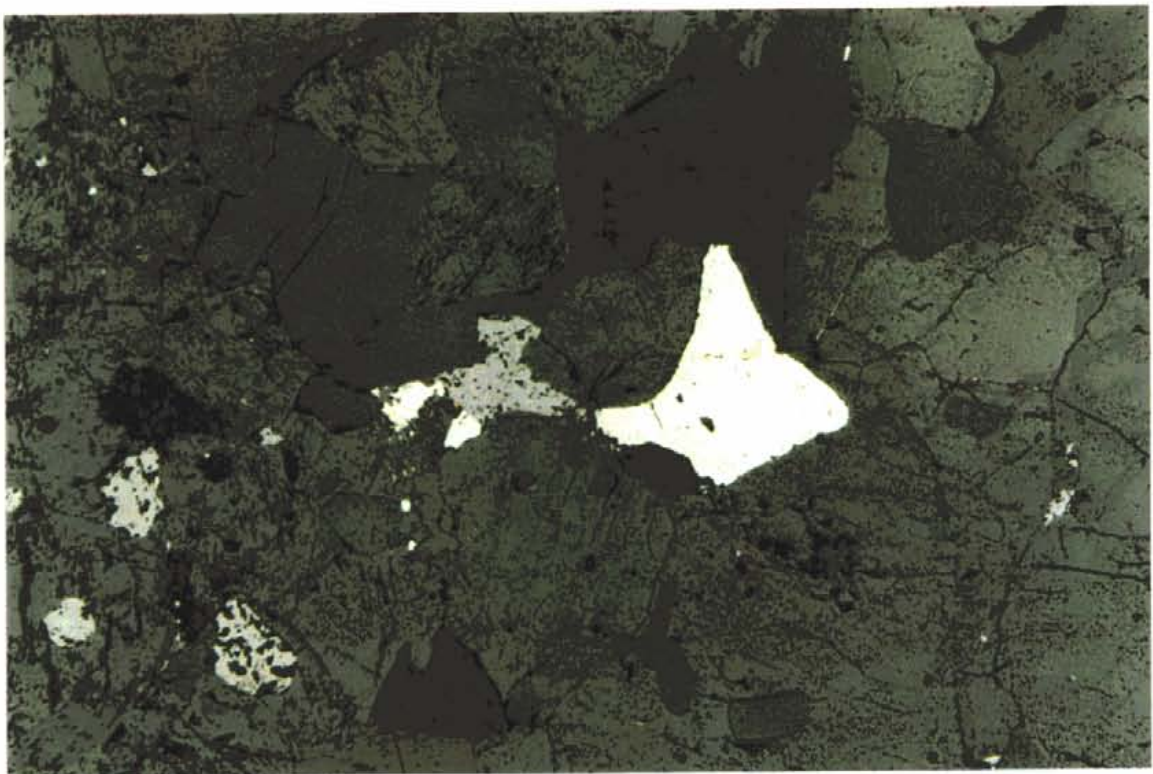
MCDDH4 - 35.4 m. Lobate aggregate of pyrite (pale yellow) and a trace of chalcopyrite (yellow). Oxide (grey) is magnetite. Reflected light. FOV = 2.6 mm.
