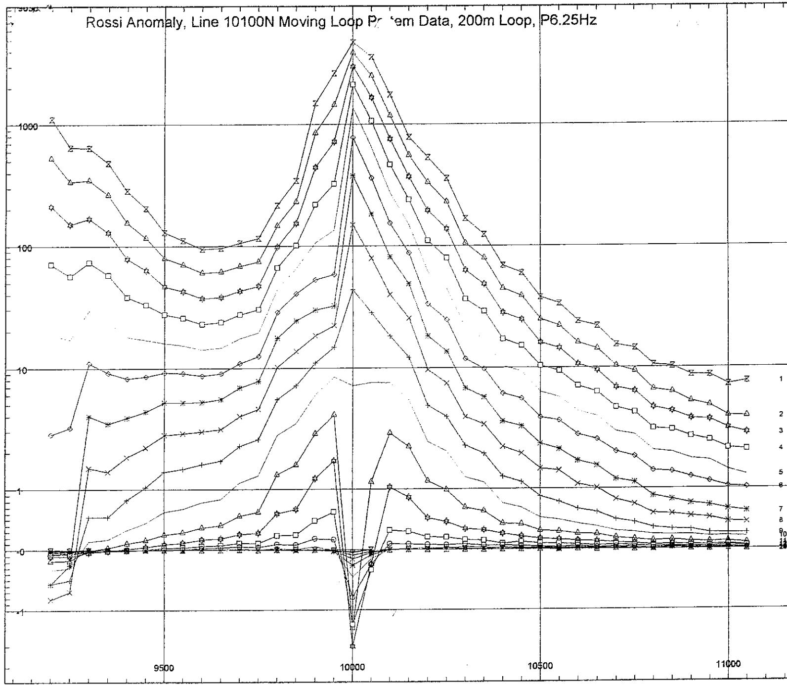
Rossi Anomaly, Line 10100N Moving Loop Problem Data, 200m Loop, P6.25Hz
