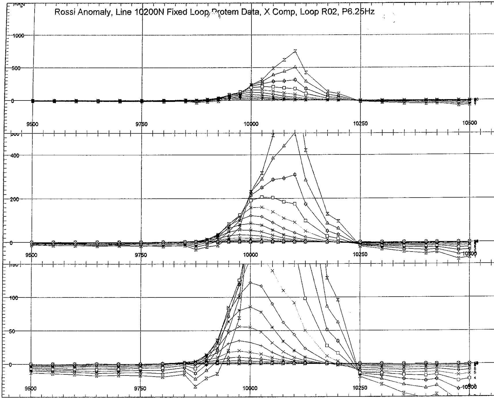
Rossi Anomaly, Line 10200N Fixed Loop, Protom Data, X Comp, Loop R02, P6.25Hz
