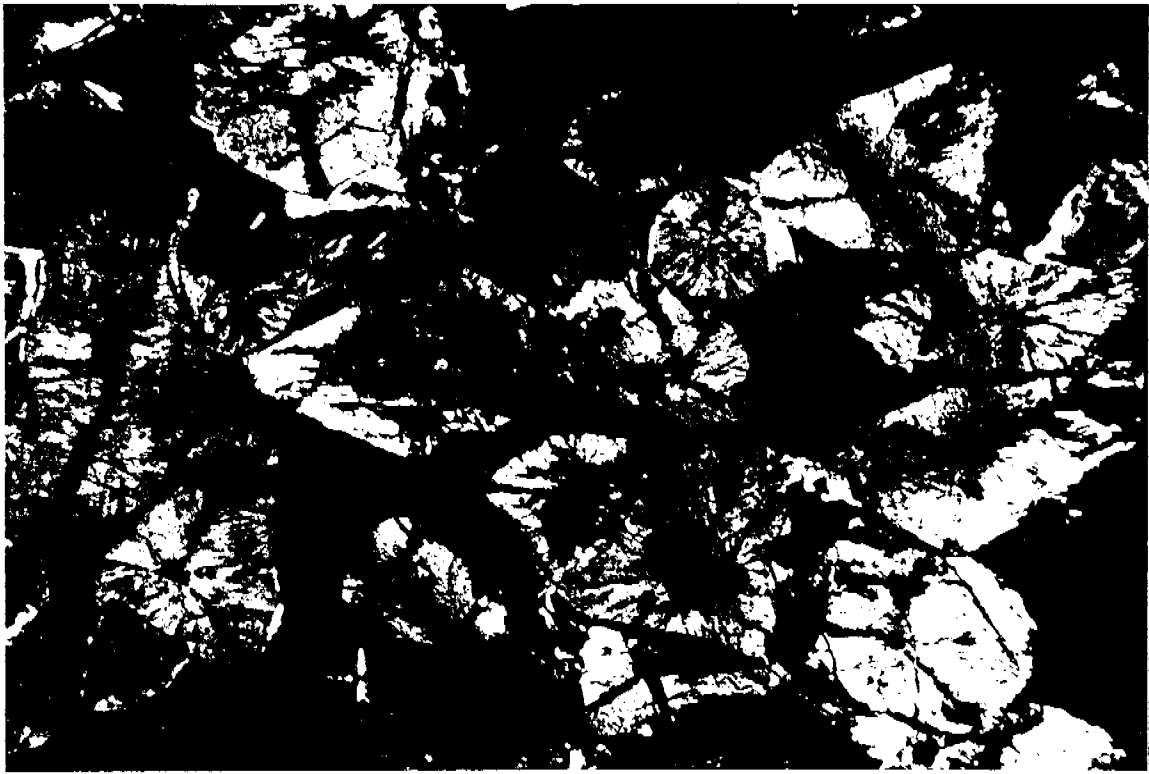
PLATE 3a: Sample MP 231 231.7 - Plane polarised light photomicrograph of an area of polished thin section MP 231 231.7 illustrating typical radial and sector zoned, relatively uniform-grained tourmaline prisms (coloured) occurring in graphite-rich laminae (black). Note the inclusion core of dusty graphite and associated radial septa emanating from the centre of the prisms. Partial fringing of the tourmaline prisms by filamentous quartz (colourless) is also shown. 4.5mm
