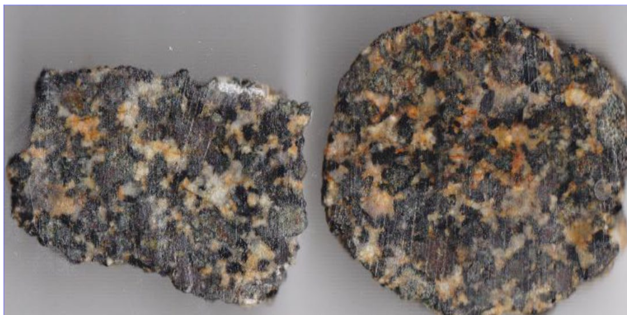
Figure 4. Photo showing 3 cm wide rock chip of lamprophyre sampled from 20LMAC046 at the Cluster target. The intrusion is not considered to have any diamond-bearing potential.
