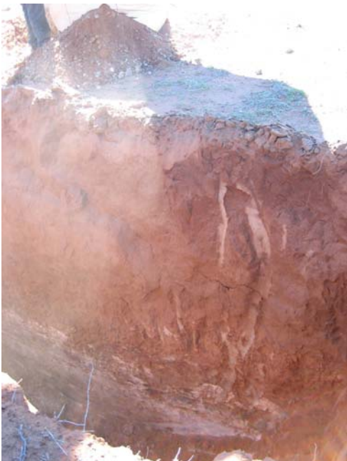
Figure 3 Photograph of Pit APBSP4 showing the calcrete at the base
