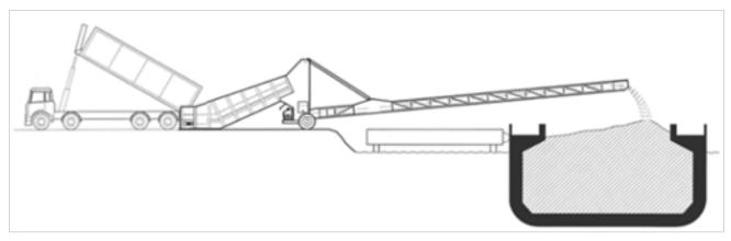
Figure 4 - Truck feeding the shiploading operation
