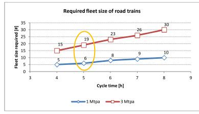
Graph 1 – Required fleet x cycle time between mine and rail
